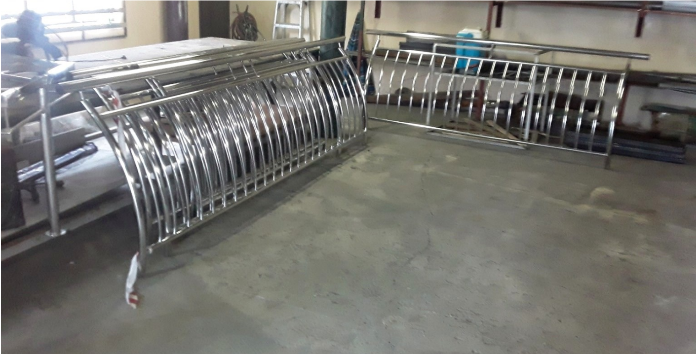
Curved stainless-steel balustrade sections
